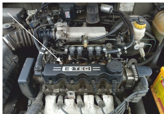
Fig. 3. Disconnecting the fuel supply to the engine cylinder of Daewoo Lanos 1.5i
