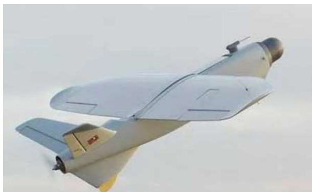
Figure 4 – Leleka-100 UAV system – a Ukrainian multifunctional unmanned aerial vehicle developed by the private company LLC “VIK DeViro” (DeVIRo TM) for aerial reconnaissance and real-time determination of precise geographic coordinates of objects [36]
