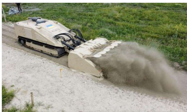
Figure – 2. Heavy demining machine DOK-ING MV-10 [33]
